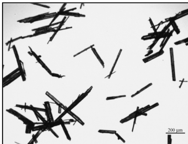
Figure 7. Microscope images of the \beta -form mannitol crystals at the end of experiment A.
